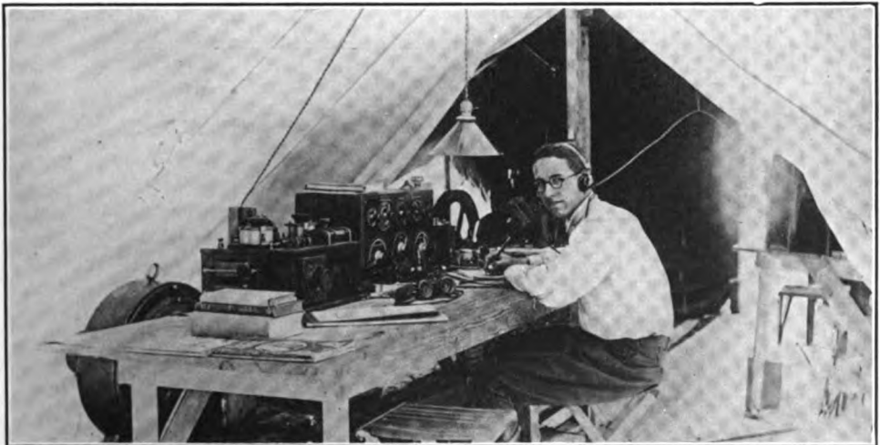
Interior of the wireless station, Lieut. Hotchkiss at key of the 2 k.w. Marconi set
